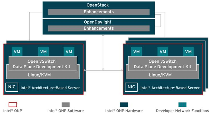
Figure 1. Intel® Open Network Platform (Intel® ONP) overview
